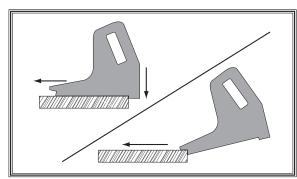
Figure 73. Side view of push block in use.
